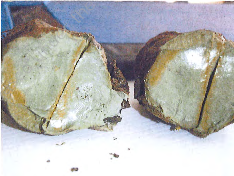
Photo 1: Polished surface and striation marks on core (MH3 8m depth)
