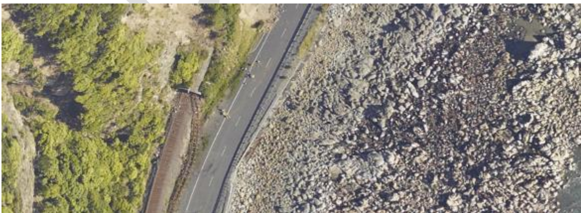
Figure 4 – Aerial imagery captured for NZ Transport Agency by AAM following the 2016 Kaikōura Earthquake identifies the rail track displacement and land uplift in the tidal area.
