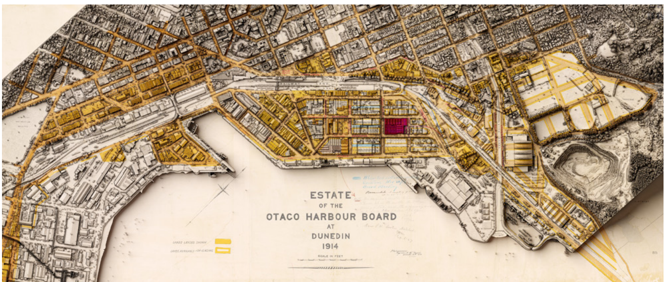
Estate of the Otago Harbour Board at Dunedin 1914, plan overlaid with LiDAR 50cm DSM. Displayed at the Survey and Spatial Conference, 2023, held in Dunedin.
